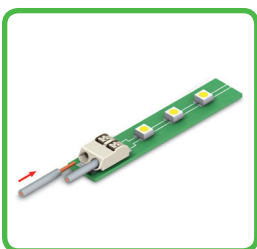
Inserting solid conductors via push-in termination.
