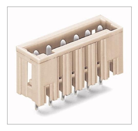
Printview: Male header (for PCBs); Press-in pin 0.6 x 0.6 mm; 4-pole; Pin spacing 3.5 mm / 0.138 in; 100% protected against mismating; with closed end; Press-in technology; Vertical PCB mounting - Item No.: 734-134/100-000
